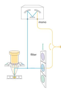
Flexibility in wavelength selection for any current and future assay requirements is best met by the MR-3942 double- monochromator with high transmission and best blocking properties for absorbance and fluorescence excitation. Use the benefits of complete absorbance and excitation spectral scans to measure wavelength shifts due to e.g. changes in pH or polarity on the chromophore's properties.
