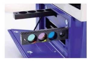
Due to their high transmission characteristics - which can be up to 25-fold that of monochromators - technologies like Time-Resolved Fluorescence (TRF) can be measured more efficiently with filters. In addition filters are available with wide bandwidths making them the ideal choice for fluorophores with wide spectra and for all luminescence based assays requiring the use of filters.
